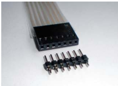
LEFT—Example of a standard flex connector with mating board-level header. MIDDLE—A 1mm pitch bare cable and mating LIF (PCB mounted) connector. RIGHT—A custom, proprietary connector system.
